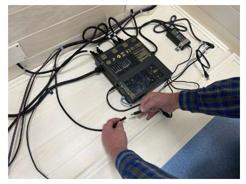
c) Connect the bundle of cables coming from the back panel to the left side of the control box.
