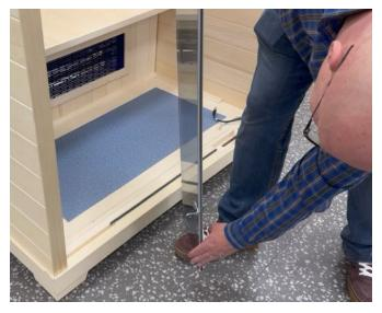
To place the side glass into the sauna, start by placing the bottom right corner of the glass in the floor panel. Then push the glass into the side panel:
