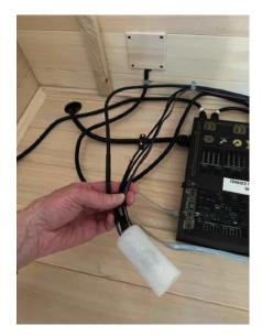
Note that 2 of the cables are similar, but one is black and the other is white. The black one connects to the receptacle labeled "RT". The white one connects to the receptacle labeled "LIGHT".
