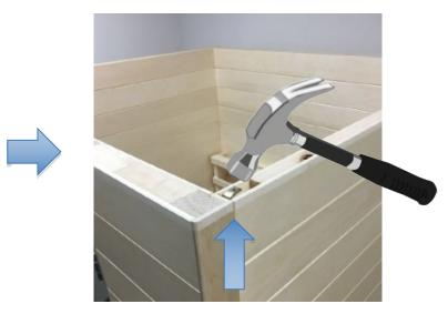
Add a screw to lock down the connection mechanism.
