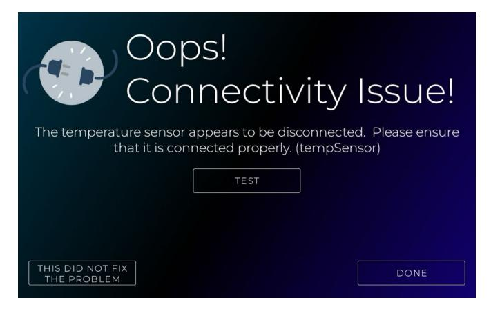
SOLUTION: Double-check that the temperature sensor connectors are securely seated.
