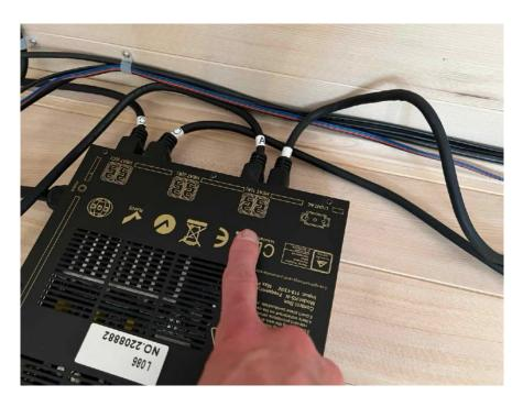
b) Connect the barrel cable between the back panel and the floor panel.
