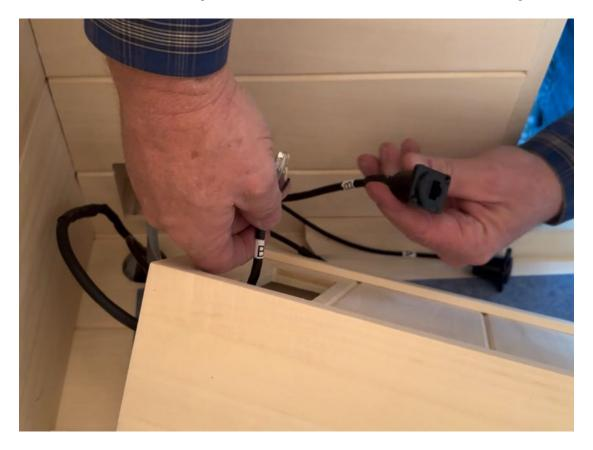
Connect the barrel cables together also through the front right heater.
