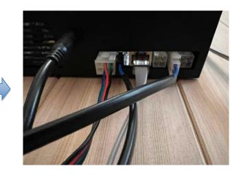
d) Connect the Ethernet cable from the floor panel to the back wall.
