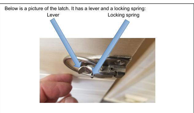
The locking spring holds the latch closed. To open the latch, place one finger on the lever and one finger on the locking spring. Then as you squeeze your fingers together, the latch will open.
