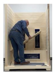
OPTIONAL: You can add 2 to 4 of the longer screws to the holes at the sides or back of the bench top to secure it in place.
