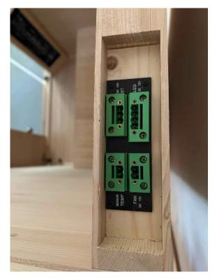
Please note that the "FAN" and temperature sensor connectors are the exact same size and could be accidentally swapped, causing the malfunction. It should look similar to this:
