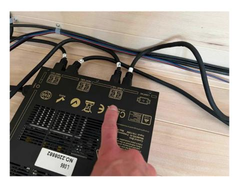
b) Connect the bundle of cables coming from the back panel to the left side of the control box.
