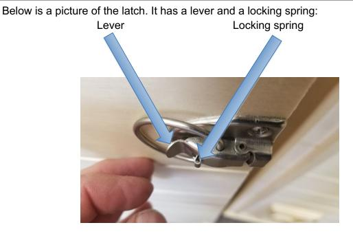
The locking spring holds the latch closed. To open the latch, place one finger on the lever and one finger on the locking spring. Then as you squeeze your fingers together, the latch will open.
