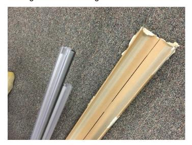
Make sure that the one you attach to the right side of the left front window has its magnet aimed outward so that the door's magnet will make contact when the door is closed. Push the magnet onto the glass starting at the top and working your way down:
