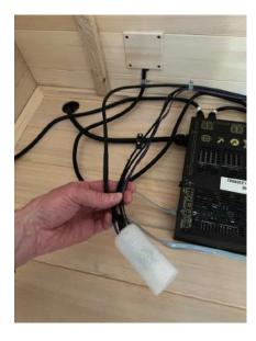
Note that 2 of the cables are similar, but one is black and the other is white. The black one connects to the receptacle labeled "RT". The white one connects to the receptacle labeled "LIGHT".
